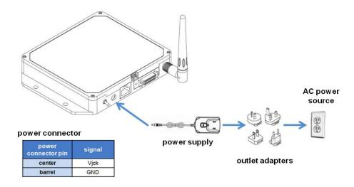
Figure 66 - Gateway Power Supply
