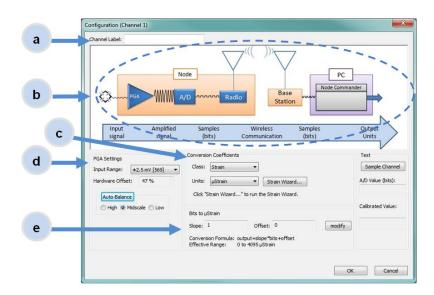
Figure 17 - Channel Setup
