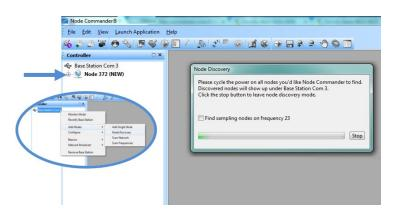
Figure 15 - Using Node Discovery
