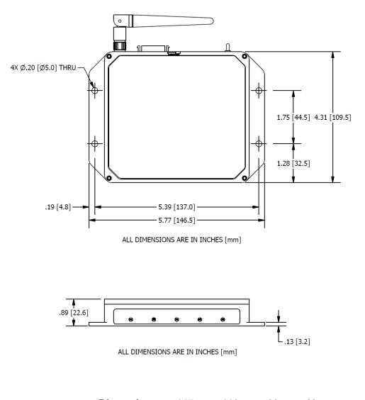
Dimensions: Weight: Enclosure Environmental Rating: 147 mm x 110 mm x 23 mm without antenna 346 grams with antenna General purpose indoor (IP67/NEMA4X rated enclosure available)
