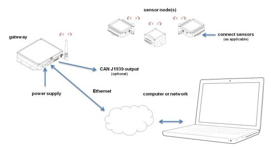
Figure 3 - System Connections
