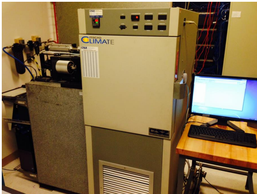
Figure 8 Fully automated calibration system including environmental chamber to applying full temperature range.
