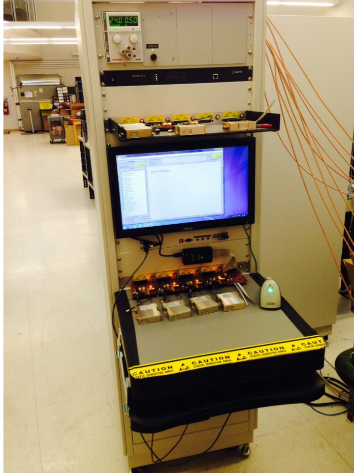
Figure 9 Functional Test Rack used to test all inertial sensors
