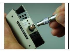
Caution!!! When removing the LEMO connector from the DEMOD-DVRT, DEMOD-DVRT-TC or DEMOD-DIN, grasp the knurled diameter and pull straight out. The lock will release and the connector will detach. Do not twist or rotate the LEMO connector.
