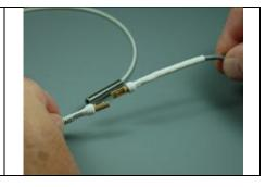
The CBL1, CBL2 and CBL25 mating cables have a 4 pin hermaphroditic LEMO connector on one end and a 4 pin keyed locking LEMO connector on the other with a red dot for alignment.
