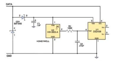
**Figure 1 Original Humidity Sensor Design**
