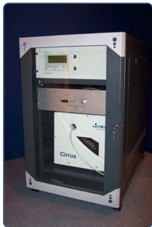
Figure 2. NDIR sensor and Cirrus™ combined to form one complete system
