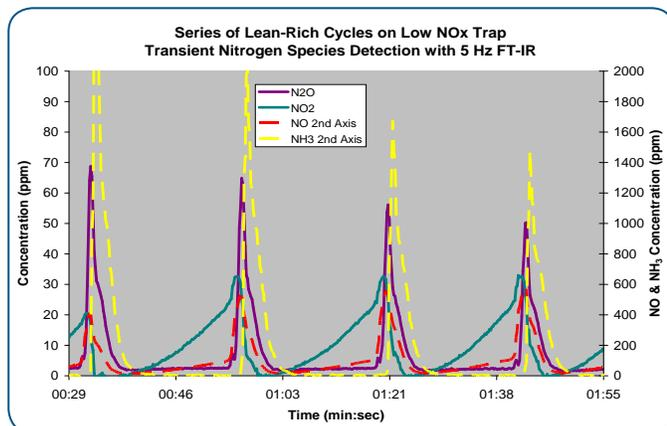
*The figure to the left shows the variability of the nitrogen combustion components during an open Lean-Rich Combustion cycle through a Low NOx Trap.*
