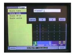
17. Using the up/down arrow keys select Scale ends and touch ENTER. You will be prompted with lo→ For this example (100 to 750°c) enter 100 for the low range of your scale and touch ENTER.
