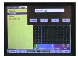
16. You should now be in the scale menu. Using the up/down arrow keys select Scale ends and touch ENTER. You will be prompted with places? (for decimal places). Using the up/down arrow keys you can select 0,1,2,3,4 or 5. For thermocouples you would only select 0 or 1. For this example select 1 and touch ENTER.
