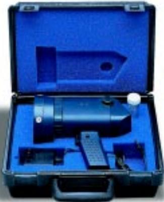
*Vibration Strobe Kit 115 includes Vibration Strobe, fast recharger, spare lamp, data collector cable and carrying case.*
