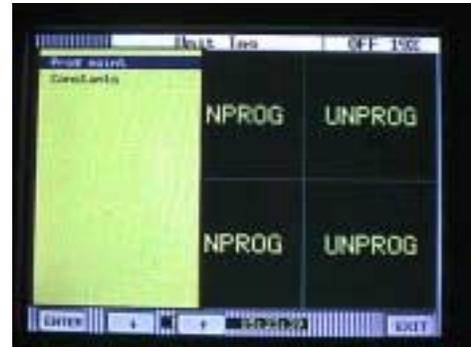
4. The numbers **1 – 9** and letters **A, B, C, D, E and F\*** will be displayed. Touch the number that represents the input or channel you wish to configure. For this example select **A** and touch **ENTER**. (**Channel A, B, C, D, E, or F must be used for totalization channels** as these channels will hold the total value in the event of a power outage. **Channels 1-9 will not**, they will reset).
