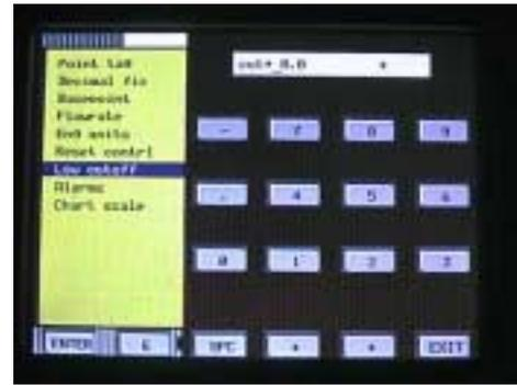
22. You should now be back in the menu beginning with Point tag. Use the up/down arrow keys to select **Chart scale** and touch **ENTER**. You will be prompted with **chart scl=** . Use the up/down arrow keys to select **A** and touch **ENTER** then touch **EXIT**.
