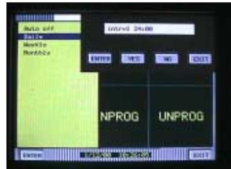
20. You will now be back at the Reset Control menu. Use the up/down arrow keys to select **Reset Print** and touch **ENTER**. You will be prompted with **print=NO\***. Touch the **YES** key then **ENTER** then **EXIT**. This enables the recorder to post the totalizer reset information to the alarm/event page. This is where you would view your daily totals.
