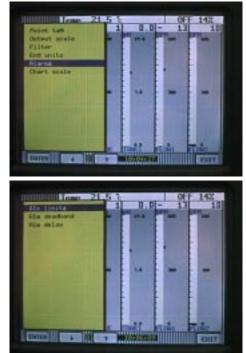
16. You will be prompted with **alarm #?** Each point has 5 internal alarm set points. You can use the up/down arrow keys to scroll select 1, 2, 3, 4, or 5. Since this is the first alarm set point for channel one, select **1** and touch **ENTER**.
