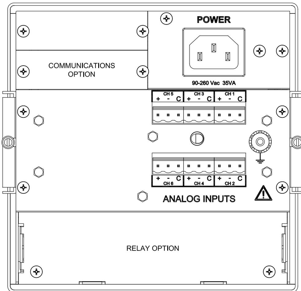
Figure 2-6 DC2000 Rear Panel Connections
