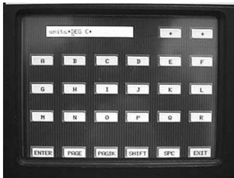
21. You have now successfully configured your thermocouple input with a non linear scale. The display will read as shown on the right. TCBO (thermocouple burnout) will be displayed until your thermocouple is connected to the rear of the unit.
