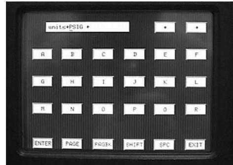
The 0-250 scale complete with **INLET** and **PSIG** should be displayed on the recorder. Use the **VIEW** button to select a particular display to verify your work.
