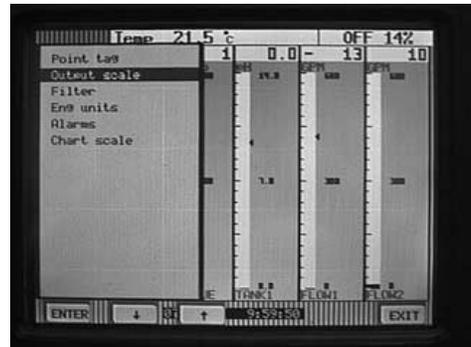
Appendix B – Configuring a 4-20 mA input to equal 0 to 150 gpm
