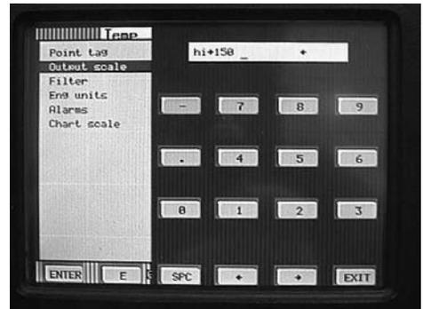
13. Using the up/down arrow keys select **Eng units** and touch **ENTER**. An alpha-numeric keypad will appear prompting you **units→ ←**. You can enter up to 5 characters. Using the **PAGE**, **PAGBK** and **SHIFT** keys, if needed, enter the desired engineering units. For this application enter **GPM** and touch **ENTER**.
