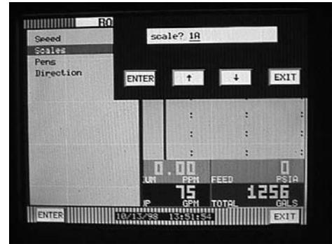
21. The scale setup menu will be displayed. Use the up/down arrow keys to select **Scale ends** and touch **ENTER**.
