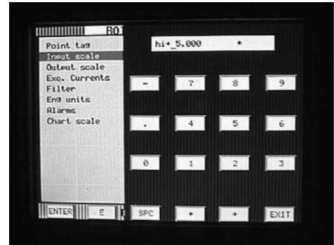
11. Using the up/down arrow keys select **Output scale** and touch **ENTER**.
