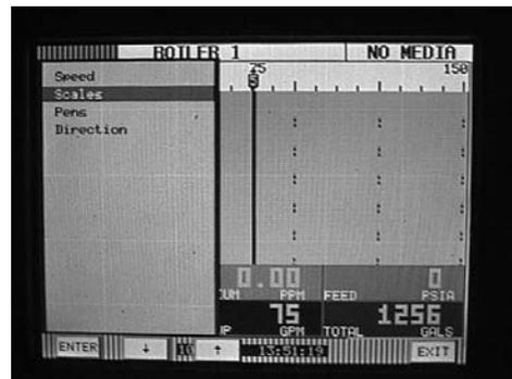
Appendix A – Configuring a 1-5 Vdc input for a 0-250 psig pressure transducer
