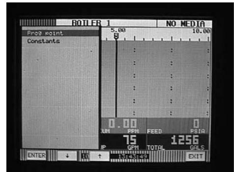
4. The numbers **1-9** and letters **A-F** represent the 15 channels that can be set up. Touch the number or letter that represents the input or channel you wish to configure. For this example use number **1** and touch **ENTER**.
