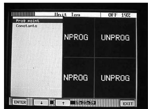
4. The numbers **1-9** and letters **A-F** will be displayed. **Channel A-F must be used for totalization channels** as these channels will hold the total value in the event of a power outage. (Channels 1-9 will not; they will reset.) For this example select **A** and touch **ENTER**.
