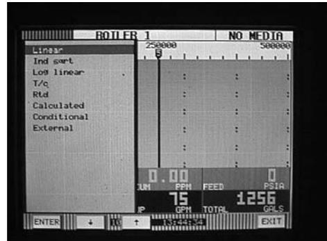
7. The menu displaying types of linear inputs should now appear. For this example use the up/down arrow keys to select **4-20 mA** and touch **ENTER**.
