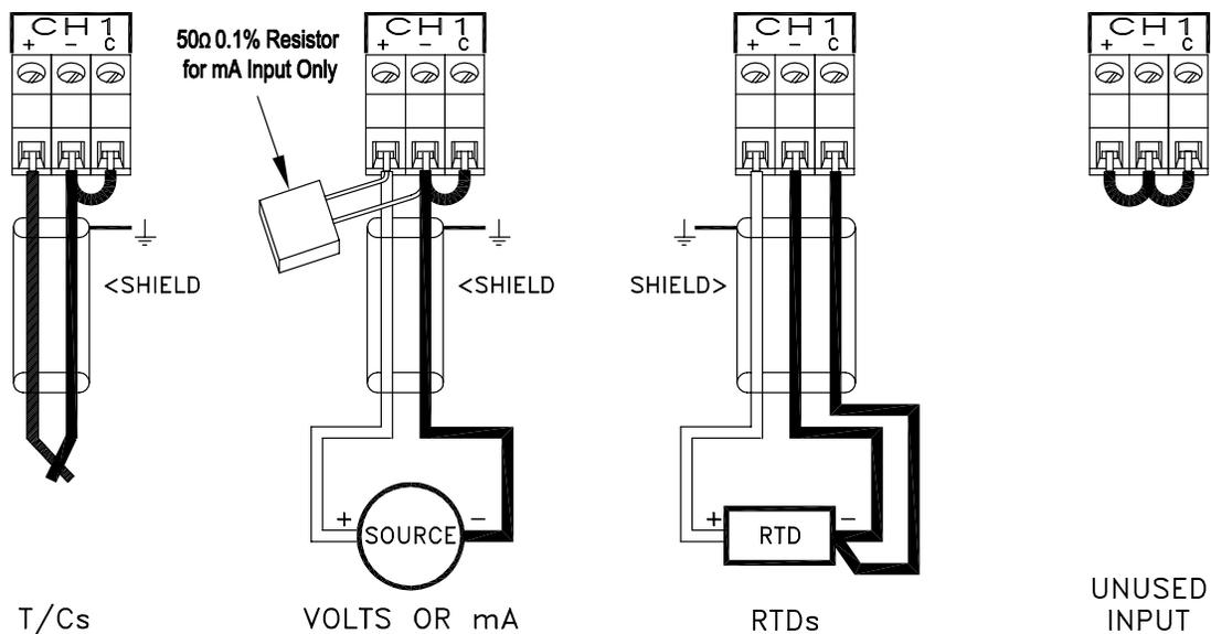
**Figure 2-7 Thermocouple, RTD and Linear Inputs**
