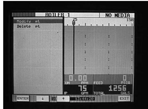
6. The menu containing types of inputs should now be displayed. Use the up/down arrow keys to select **Linear** then touch **ENTER**.
