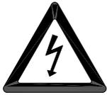
**Signal input connections. Hazardous potentials may exist on signal input terminals which are floating with respect to case ground. These hazardous potentials may be on the rear terminal panel of your instrument. Any voltage potential at the signal source will exist on the instrument's respective signal input terminal (i.e. power generator stator winding).**
