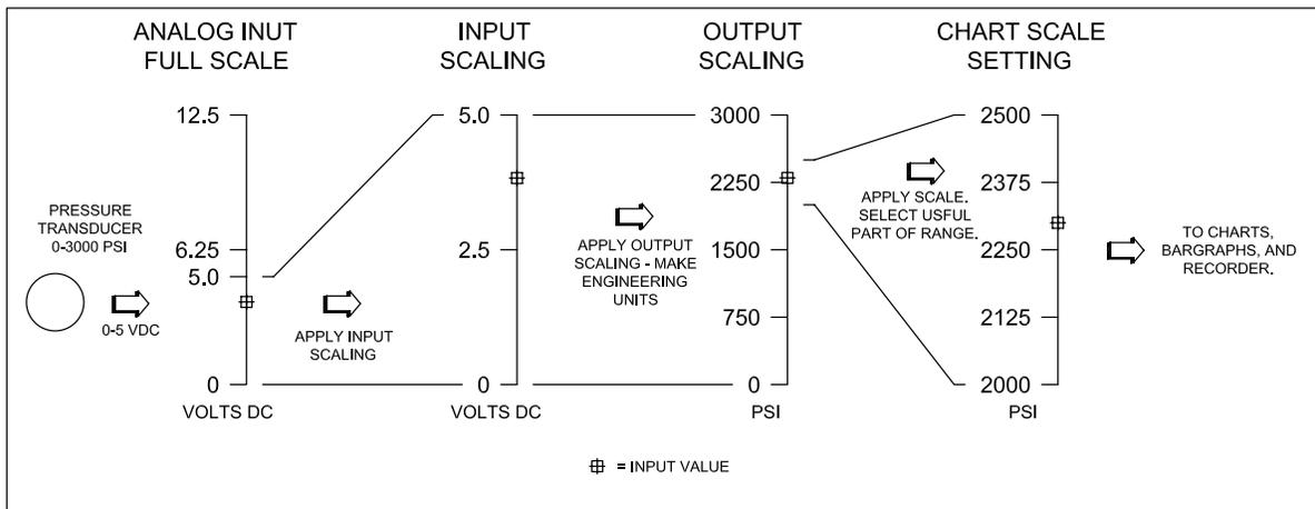
Figure 3-14 Scaling Example
