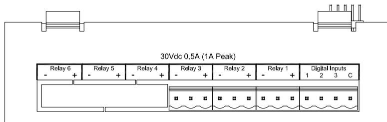
Figure 2-9 Solid State Relay Connections (3 Channel Shown)
