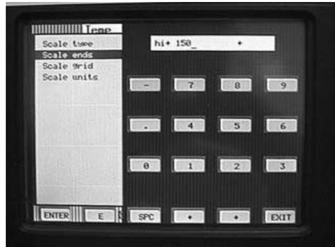
29. The 0-150 scale complete with EFFLUENT and GPM should be displayed on the Recorder. Use the VIEW button to select a particular display to verify your work. You will also notice that your high alarm set point is marked at 120 with an arrow.
