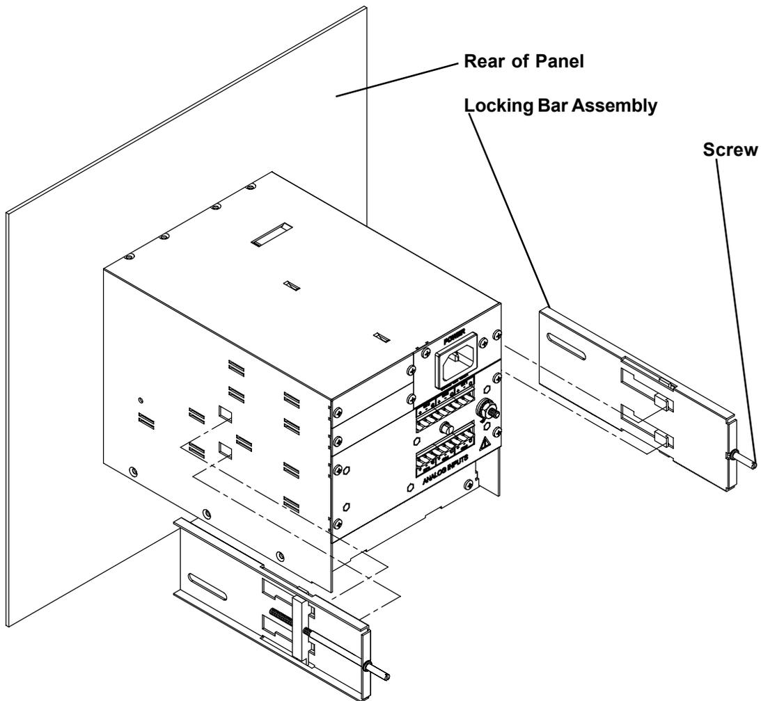
**Figure 2-3 Rear View Panel Installation**
