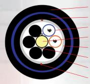
Black PE Outer Sheath Black Polyethylene Inner Sheath Loose Tube With Fibres & Gel Central Strength Member Core Wrapping & Strength Member WS Yarns Blue Polyamide Intermediate Sheath Ripcord(s)
