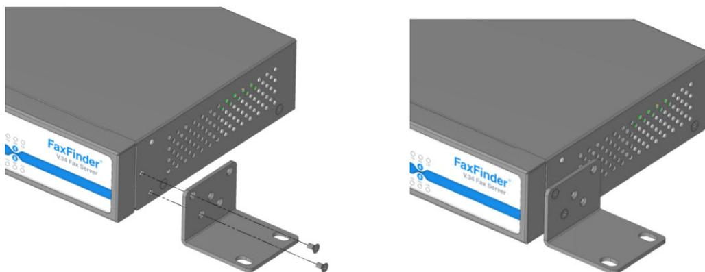
2. Secure the bracket to the device using two provided screws.
