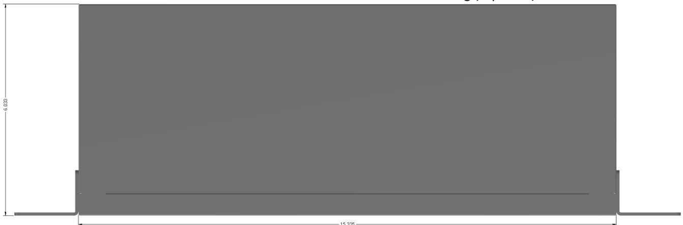
Dimensions with brackets attached for rack mounting (front view)
