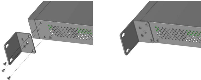
2. Secure the bracket to right side using three provided screws as shown.
