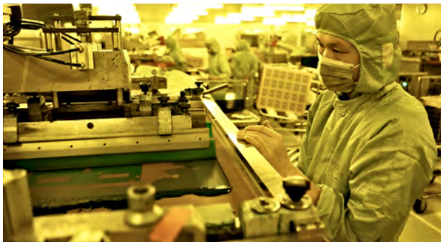
A screen print station in the clean room at Suntak, Shajing. UL has an open database on the internet where visitors can search amongst approved PCBs, laminates and surface treatment materials.
