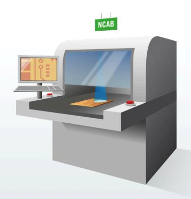
Inspection of the circuitry against digital 'images' (based upon data) to verify that it is free from such defects as shorts, opens, etc.
