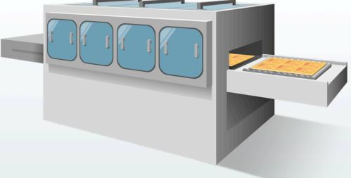
Removal of the remaining dry film (blue), etching of the unwanted & exposed copper and tin - leaving the copper (under the tin) that defines the circuitry.
