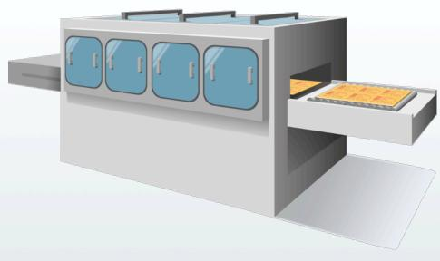
Removal of the unwanted copper (**not** protected by film) from the panel through etching, to leave copper circuitry that matches the image.
