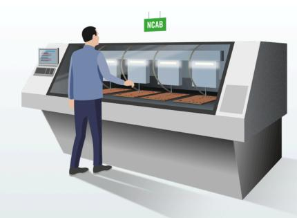
Mechanical drilling of holes to facilitate the provision of electrical continuity between layers. At this moment, the barrel of the hole has NO metallic deposit.
