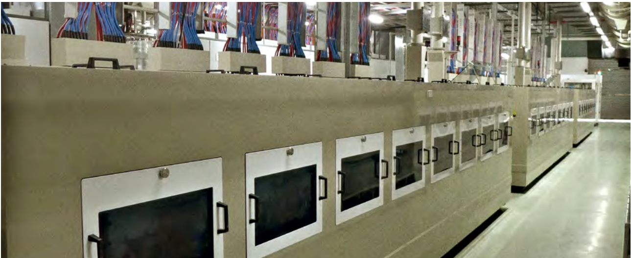
A horizontal plating line used for copper filling of micro vias on HDI product.
