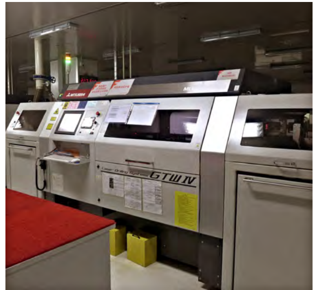
The laser drill is used in HDI production.
