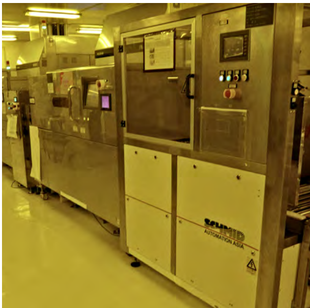
A Laser Direct Imaging (LDI) machine transfers and prints the pattern directly onto the circuit board material by means of laser beams.
