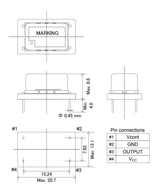
Dimensions in mm Tolerance +/-0.2
