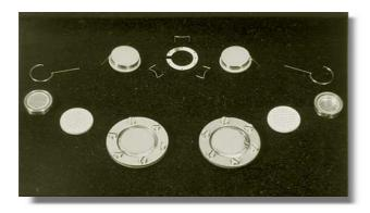
sists of a membrane, back electrode and delay plate. The two capsule halves are mounted together back-to-back with a distance foil, thus forming a dual membrane capsule, similar to the proven M 7 capsule from U 47, U 48 and M 49 fame, but considerably smaller.
