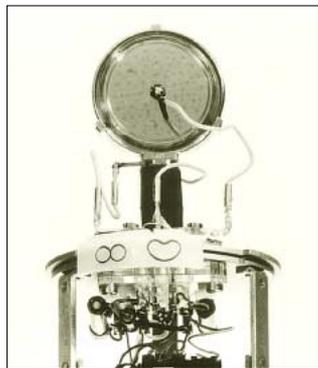
Both capsule halves thus act as a cardioid capsule and led Neumann to make the rear membrane electrically active by coating it with gold too. When connecting both cardioid halves in parallel, the capsule produces an omni directional pattern. If only one membrane is connected, the microphone works as described above as a cardioid.
