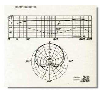
brane at the same instant that the sound travelling around the side strikes the front. Ideally, the resulting forces cancel at the membrane and do not produce any output. In this way, a cardioid directional characteristic is achieved.
