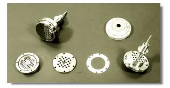
of the membrane has been removed to expose the back plate electrode. The diagrams in the bottom row show (from left to right) the back plate electrode with the contact spring inside (rear view), the delay plate, the distance ring and the capsule holder with the rear sound inlets. Above right we see the cover with a fine wire mesh in the middle.
