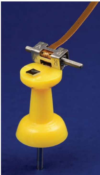
Figure 1. SQL piezoelectric motor and NSD-2101 drive ASIC on a pin.
