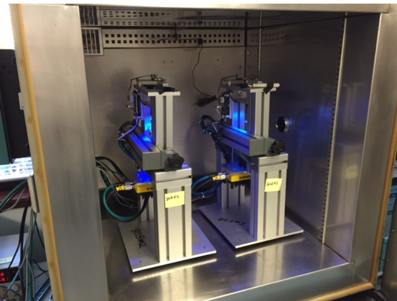
Figure 10: Two Cobra positioners in 400,000 cycle life test using ST80B in temperature chamber.
