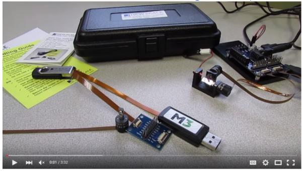
The two-axis beam steering system and one-axis mirror positioning system developer's kits include demo boards and USB connection for easy evaluation using New Scale Pathway software on your PC. Watch the video (3:32)
