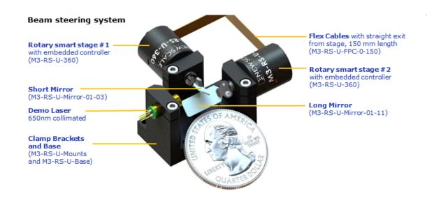
Patented piezoelectric motors along with position sensors, bearings, drive electronics and embedded firmware are all integrated into each miniature rotary stage. The positioner accepts direct input of high-level digital motion commands from a system processor via I2C, SPI, UART or analog servo interface.
