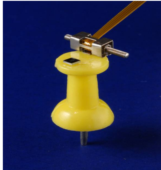
Fig. 3: Smallest SQUIGGLE motor with NSD-2101 ASIC Driver
