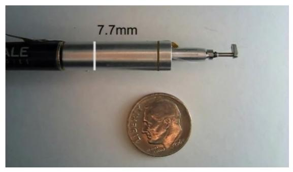
See the Cobra fiber positioner in operation, along with an animation showing how it achieves full coverage of an 9.5 mm diameter fiber patrol area with an actuator spacing of 8 mm in an array. Watch the video (2:52)
