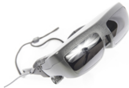
eSight eyewear for people with low vision incorporates New Scale's M3-F focus module with a high-resolution video camera and two displays.
