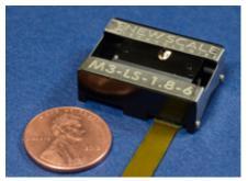
M3-LS Linear Smart Stage has integrated drive electronics for smallest size, fast and simple system integration.
