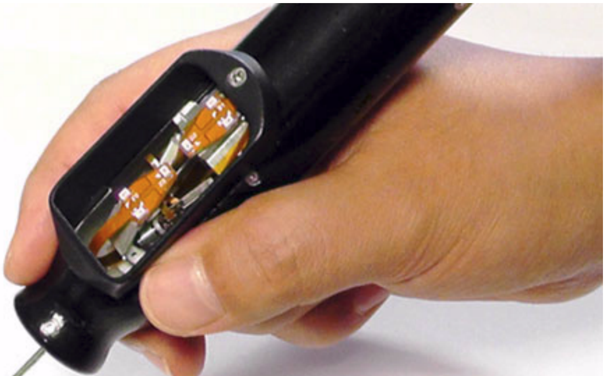
World's smallest hexapod positioner in a handheld surgical tool (Carnegie Mellon University)
