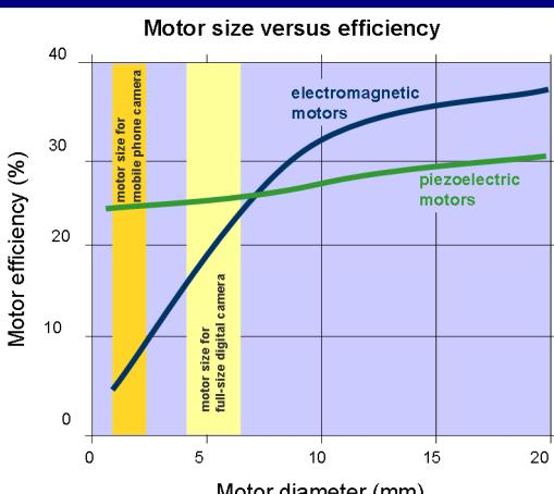
**Piezoelectric motors are scalable** – Unlike electromagnetic motors, SQUIGGLE motors retain their efficiency as size decreases.
