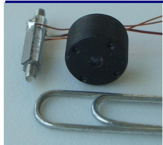
A tiny SQUIGGLE motor (4 mm diameter) is shown next to a phone camera lens. The patented piezoelectric motor uses ultrasonic vibrations in a threaded nut to directly rotate a mating screw, producing precise linear motion.
