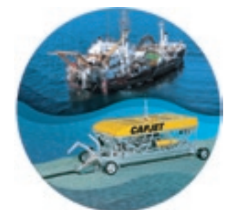
Capjet burying equipment in operation
