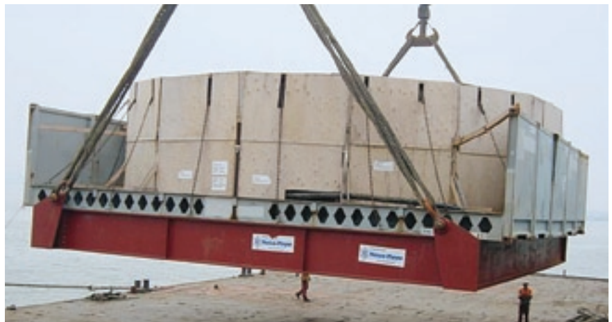
Loading of a flat containing 300 tons of submarine cables for China
