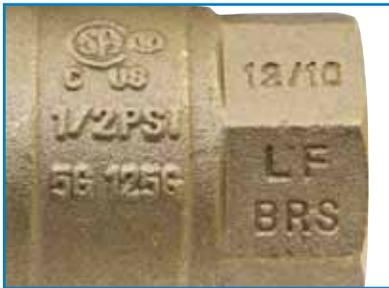
Lead-Free fittings and valves not manufactured from Performance Bronze™ are cast with an “LF” in the body
