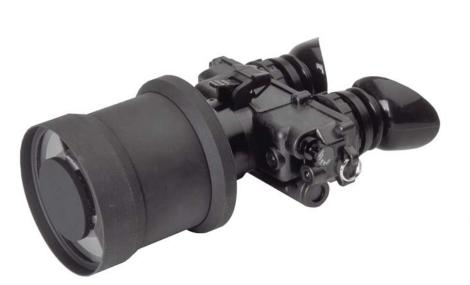
**ANVS-2347** long-range night vision binocular is built around standard AN/PVS-7 body and 5x catadioptric objective lens. It was specifically designed to meet the long-range observation needs of military and law enforcement personnel. It has a far better performance compared to a 5x afocal lens attachment often used to convert PVS-7 to a long-range binocular. ANVS-2347 is an ideal tool for covert surveillance, border patrol and spotting in low light conditions. Covered by oneyear warranty.
