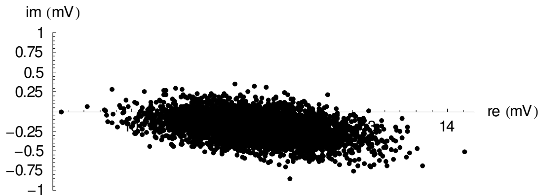
Figure 5-12. 5000 realizations of the real and the imaginary value of the spectrum at 4 GHz (maximum negative correlation \cong -0.4 ).
