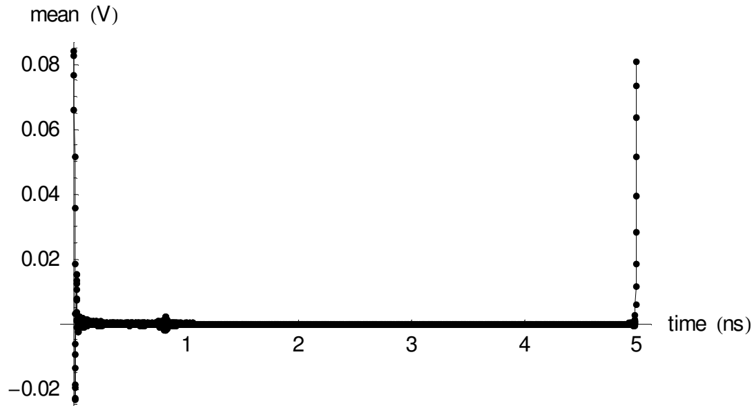
Figure 5-1. Sample average of the impulse response disturbed by jitter noise.
