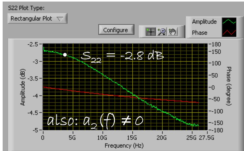
$$\underbrace{b_2(f)}_{\text{LSNA}} = \underbrace{S_{21}(f)}_{\text{VNA}} \cdot \underbrace{a_1(f)}_{\text{LSNA}} + \underbrace{S_{22}(f)}_{\text{VNA}} \cdot \underbrace{a_2(f)}_{\text{LSNA}}$$
