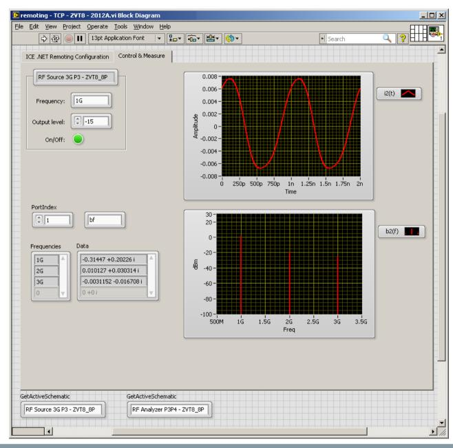
Setting the frequency and output level of the RF source based on the unique name assigned in ICE
