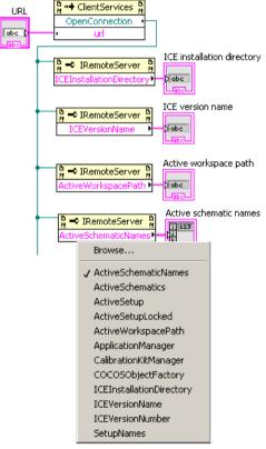
LabVIEW allows to select the desired property or method of the IRemoteServer which is returned when opening the connection at the specified URL
