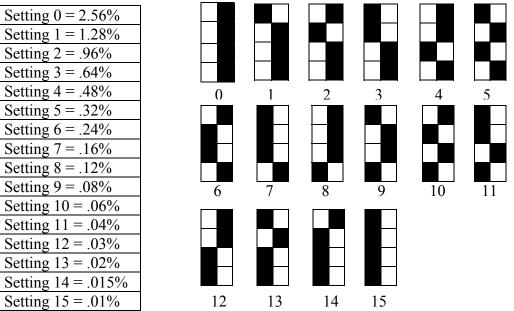
Sensitivity DIP switch positions (shaded area).
