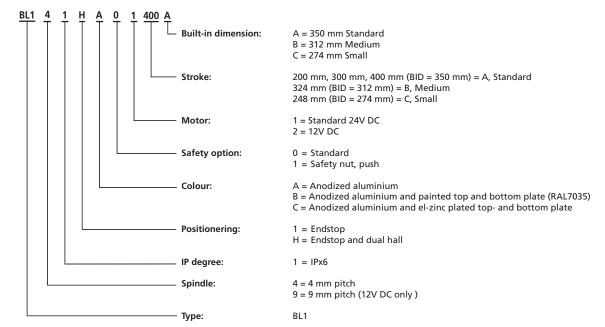
Note: Please note that it is not necessary to choose the "safety nut" in order to comply with applicable standards. The BL1 lives up to applicable standards without the "safety nut". It can of course be chosen as a USP or KSF.
