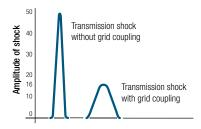
This unique characteristic is due to the torsional flexibility of the coupling being proportionate to the unsupported length of each flexible grid rung. The resultant reduction in peak loading protects and extends the life of the transmission equipment.
