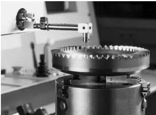
Computerized mapping of gear tooth profile
