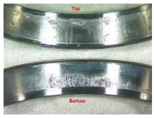
Examples of tapered roller bearings showing water contamination and misalignment damage.
