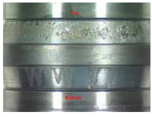
Examples of tapered roller bearings showing water contamination and misalignment damage.
