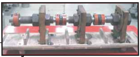
Fig. 4: Head with three mounted test bearings
