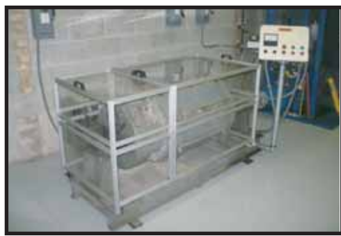
Fig. 2: Rotating Drum Test Stand
