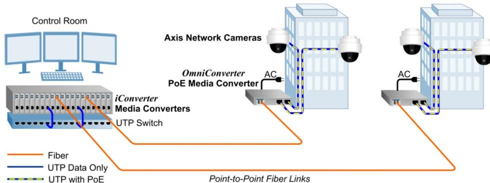
In this application, Axis network cameras are deployed on buildings. At the Control Room, fiber is distributed from a copper Ethernet switch using a high-density chassis of iConverter media converters that provide reliable fiber connectivity and preserve the investment in the existing switch equipment.
