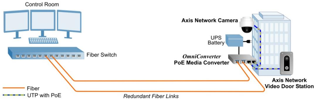
In this application, an Axis network camera and an Axis Network Video Door Station are deployed on a building in a large, high-security complex. Redundant fiber links are distributed from a fiber switch in the Control Room.
