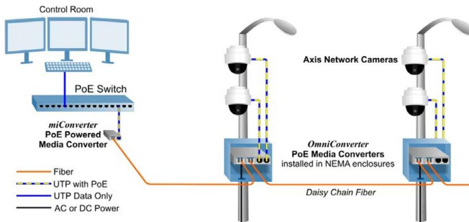
In this application, Axis network cameras are deployed on light poles along a city street. At the Control Room, fiber is distributed from a PoE switch using a miConverter PoE powered media converter that draws power from the PoE switch and eliminates the need for a separate power cable and adapter.
