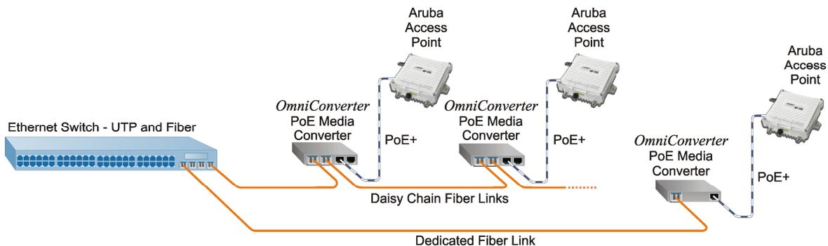
In this application, fiber optic cabling originates from a fiber port on the Ethernet switch, and connects to a fiber port on an AC or DC powered *OmniConverter* media converter, located near the access point or mesh router. The *OmniConverter's* 10/100 or 10/100/1000 UTP ports are connected to access points or mesh routers using up to 100 meters of Cat5 or better LAN cabling, as required, and provide both power and an Ethernet link across this single medium.
