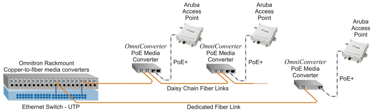
In this example, no fiber ports are available at the Ethernet switch. Rack mounted copper-to-fiber media converters are used to create the fiber interface. Rack mounted media converters can provide up to 19 media conversion ports in less than 2U of rack space. For low density applications, standalone media converters may also be used.
