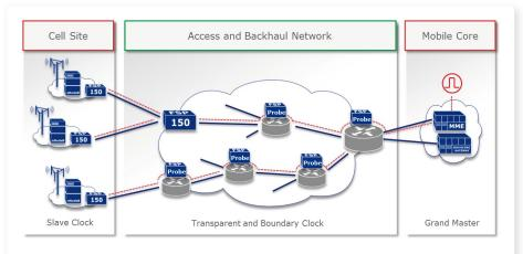
Figure 3: Enabling existing infrastructure with probe devices
