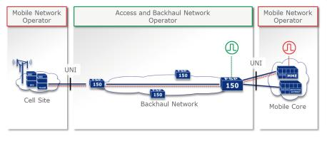
Figure 1: Multi-operator mobile backhaul environment
