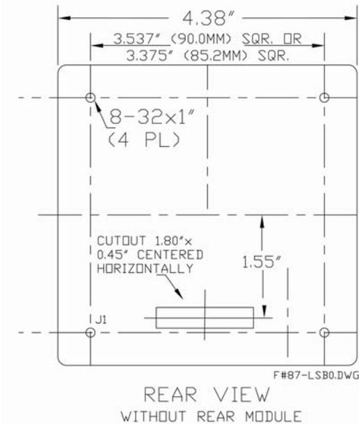
2) Use the included hardware (4 locknuts, plastic spacers and washers) to secure the unit to your panel in the following manner:
