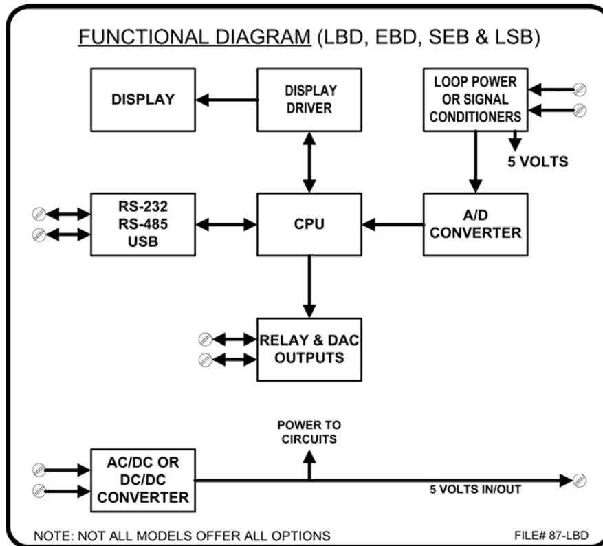
Figure 1: A simplified internal structure of the controller
