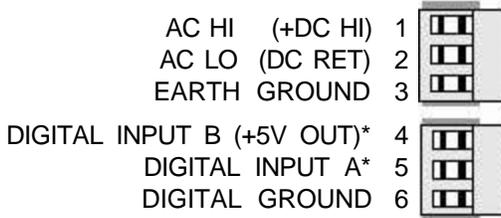
\*Note: Non-isolated digital control inputs A and B are menu selectable for Tare, Peak Display, Hold, or Reset and external control of decimal points.
