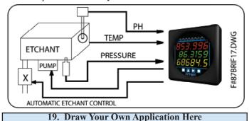
Note: Above typical applications use the HI-Q126 as the controller, but they also apply to most any HI-Q series controllers.
