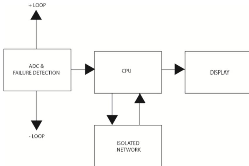
Figure 1: Block diagram of Powerless™ NTM component interactions
