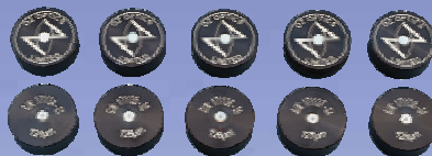
Pin Gauges for Fiber OD Measurements
