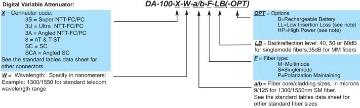
Note 1: LL ≤ 0.6 dB with units that have 60 dB return loss and fiber core of at least 5 microns.
